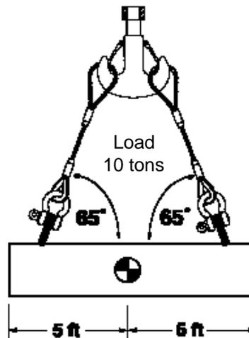
In this example the 10 ton load is equally centered between the pick points but we lift at a sling angle of 65°. We know that each sling is subjected to 5 tons VERTICALLY. In applying the calculation from the previous section (Angularity) we arrive at
