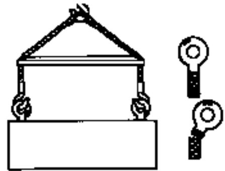
We recommend that eye bolts only be used at a horizontal angle greater than 45°. Sling strength at 45° is 71% of vertical sling capacity.
