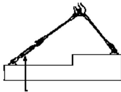
If you lift an off-center load the sling leg can be fitted with a turnbuckle to level the load. Instead of a turnbuckle you may use a come-along but be sure the capacity fits the job.
