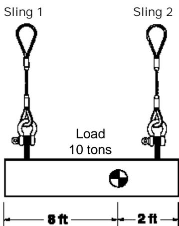
When the center of gravity is not equally spaced between the pick points, the sling and fittings will not carry an equal share of the load. The sling connected to the pick point closest to the CG will carry the greatest share of the load.
