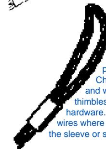
Inspect the bearing point of the eye. Check for deformation and wear of sleeve, thimbles, and all attached hardware. Check for broken wires where the rope enters the sleeve or socket.
