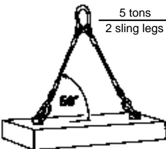
$$\frac{5 \text{ tons}}{2 \text{ sling legs}} \times \text{AF } 1,305 = 3.26 \text{ tons}$$
