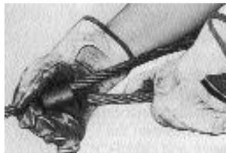
The rope is 'looped back' into a sleeve (steel or aluminum) which is swaged to form a permanent load bearing bond between the two rope parts.
