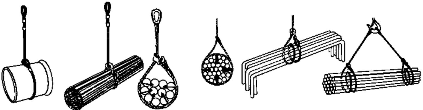
Standard choker hitches provide better load control as long as the loads are short. When lifting longer bundled loads there is the danger that some of the bundle content may slide out of the sling. As can be seen, a standard choker hitch compresses the load from three sides only
