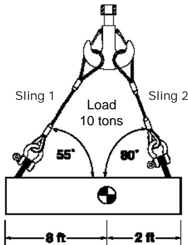
From the calculation on the left we know that sling 1) is tensioned to 2 tons, and sling 2) is tensioned to 8 tons. However both slings are on an angle, hence we must apply the angularity factor for EACH sling:
