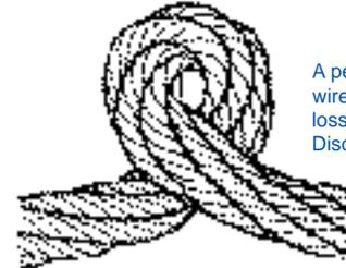
A permanent kink in a wire rope sling causes loss of strength. Discard the sling !
