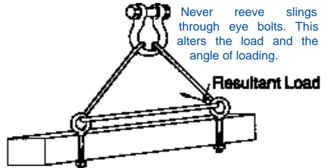
Use swivel hoist rings for rigging. They self adjust to any load angle and CROSBY® hoist rings are clearly marked with their capacity and recommended torque values.
