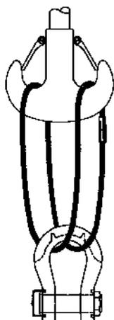
Use large enough hooks AND large diameter shackles to avoid crushing and kinking of the sling.
