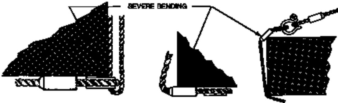
Do not place the splice sleeves, rope thimbles, or sling hooks around corners. A sleeve failure under these condition will result in the failure of the sling and you WILL drop the load. Check the sleeves regularly for nicks and cracks. Rope sleeves are NOT designed to be hooked under loads and be used as a swaged button; rope sleeves secure the rope ends and are not intended to lift the load. DO NOT WELD ANYTHING ONTO THE ROPE SLEEVE OR TO ANY ROPE END ATTACHMENT.
